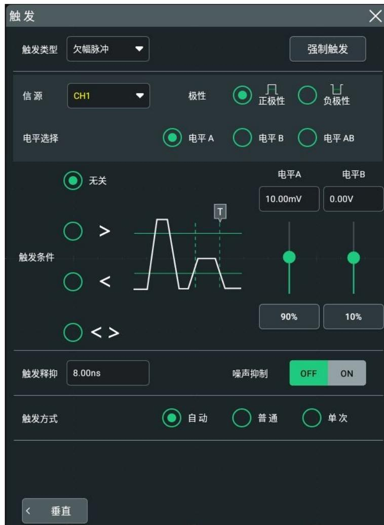
图 8.16 欠幅脉冲触发配置菜单
