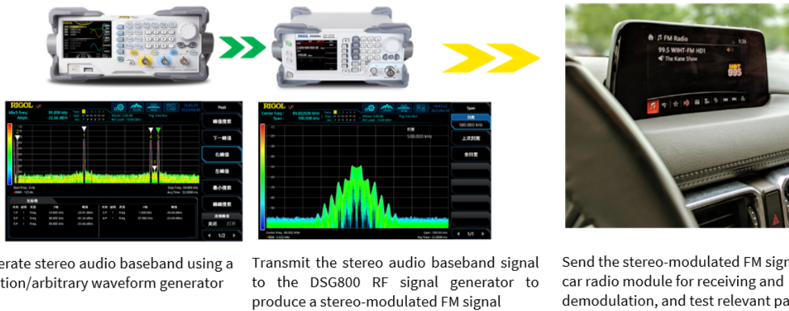
Figure 6. FM Stereo Generation Scheme for R&D Testing Phase
