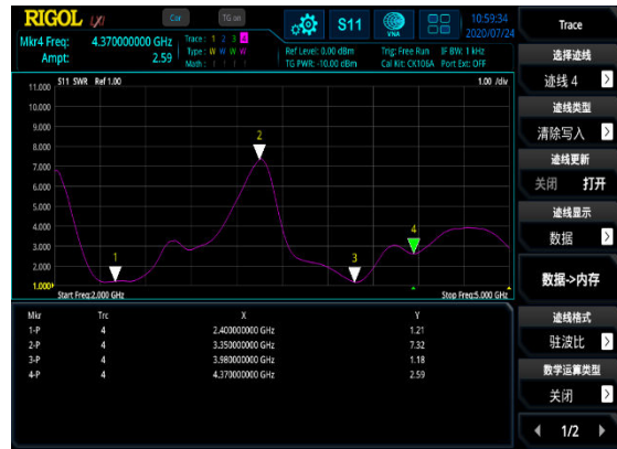
Figure 4.6 RSA5065N VNA Mode for VSWR Test of the Antenna
