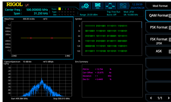
Figure 4.2 RIGOL Spectrum Analyzer Performs Signal Demodulation and Analysis
